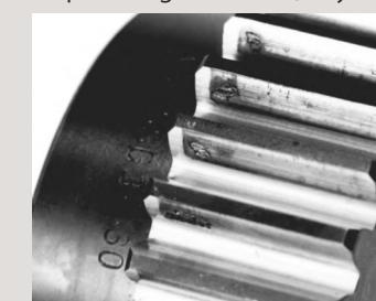
Poor tooth contact and pitting
